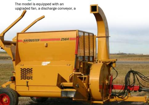
The machine handles two bales at once: it carries one round bale in the chamber and the second one on the loader. Both vertical and horizontal adjustment is hydraulically driven, which allows to position the bale from the tractor cab. The 2564 Model is suitable for a wide
